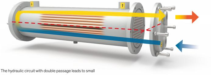
I he hydraulic circuit with double passage leads to small dimensions with the same thermal performance. For easy installation, the cooling water inlet and outlet connections for the water-glycol mixture are located on the same side.
